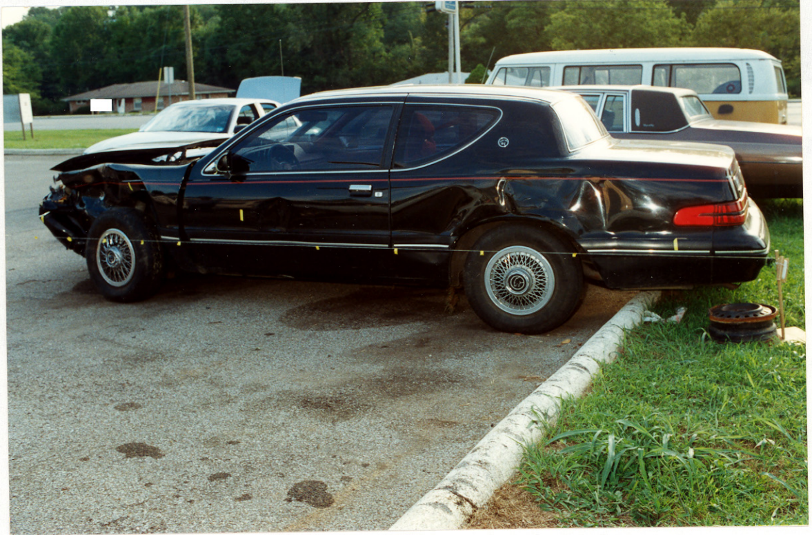
112. Left side view of the secondary (side slap) damage.
